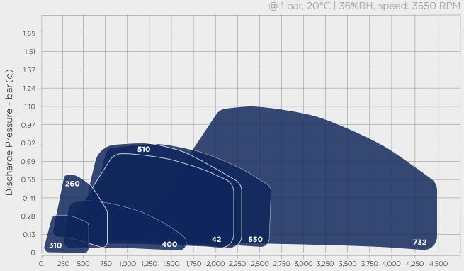
Inlet Volume Flow Rate - m³/h
